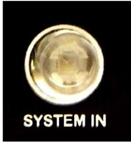
**SYSTEM IN** switch in OFF position all Encode/Decode processing is by-passed.
